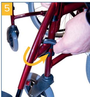
To remove the leg support, swivel it about 45° outwards and pull it upwards. To replace the leg supports, insert them at an angle of about 45° and then swivel them inwards until they click into place.
